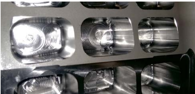
Ti17 pocket machining with dynamic tool path
