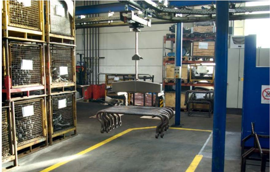
**2** Anti-roll bars for the commercial vehicle and track vehicle industry are one of Beinbauer's main product lines and account for 14 per cent of the company's turnover (photo: Hanser)
