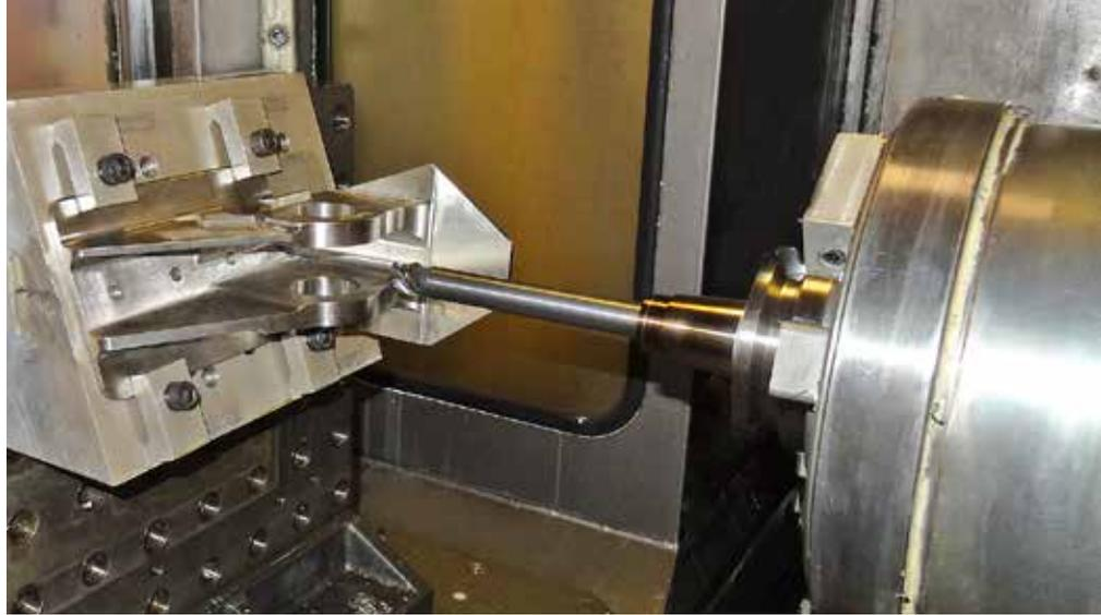
Brace machined by Mitsubishi Materials iMX exchangeable head end mills
