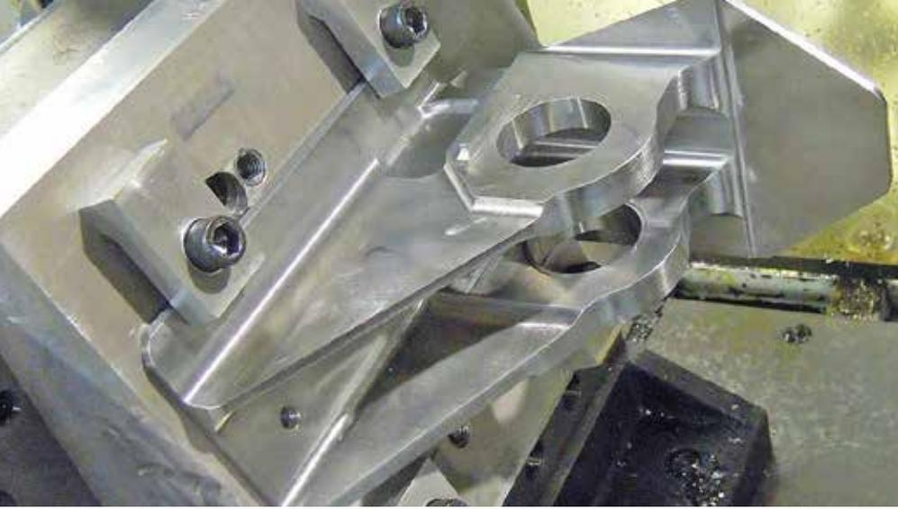
Brace made of TA6V (Ti-6Al-4V)
