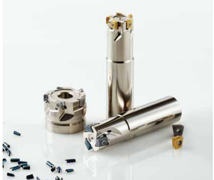
smaller machines. The 200 series has 09 size inserts, whilst the 300 has larger 12 size inserts and both series are available in shank, screw-in and arbor types, ranging from Ø16 - Ø80.
