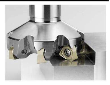
Furthermore, a high maximum depth of cut of up to 8.2mm enables efficient shoulder milling capabilities. In order to meet component surface finish expectations, the bottom of all inserts feature a large radius geometry that acts like a traditional wiper.
